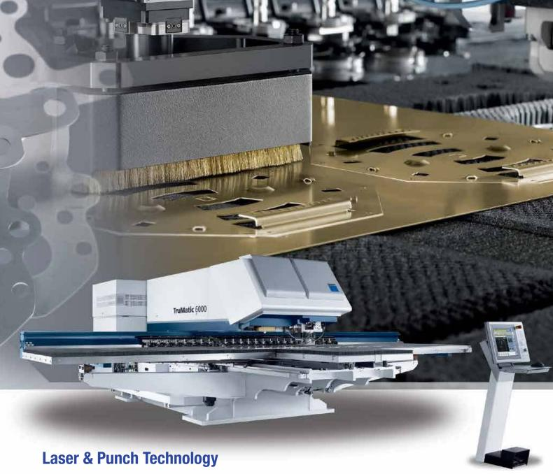
The "combo" is a versatile machine with sophisticated laser and punching technology. The powerful punching head and laser guarantee high turnaround and excellent quality. For sensitive materials, which must not have any scratches underneath, we use brush tables combined with the descending die.
